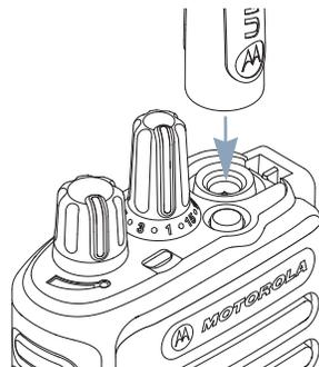
To remove the antenna, turn the antenna counterclockwise.
