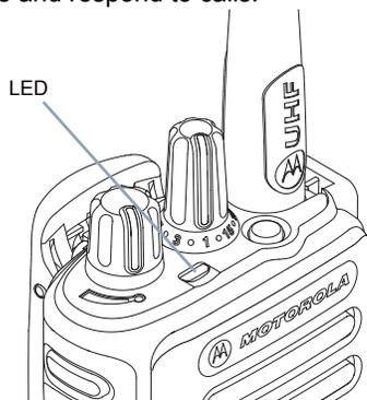
*The LED lights up solid green while the radio is transmitting and blinks when the radio is receiving.*
