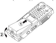
2 To attach battery cover, align it in place and slide the battery latch until it snaps into place. Slide battery latch into lock position.
