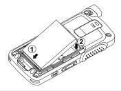
2 To attach battery cover, align it in place and slide the battery latch(A) until it snaps into place. Slide battery latch into lock position.
