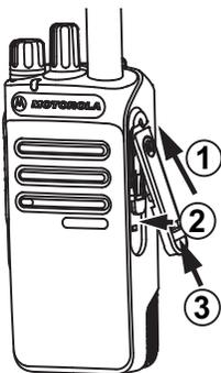
Insert the slanted end of the cover into the slots above the universal connector. Press downward on the cover to seat the dust cover properly on the Universal Connector.
