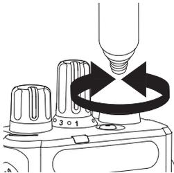
*To remove the antenna, turn the antenna counterclockwise.*
