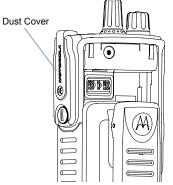
Insert the hooked end of the cover into the slots above the universal connector. Press downward on the cover to seat the lower tab properly into the RF connector.
