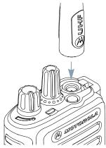
To remove the antenna, turn the antenna counterclockwise.
